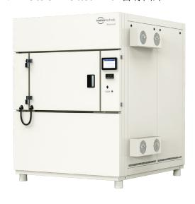
With the Damper Shock, weisstechnik is expanding its portfolio of temperature shock test chambers. The Damper Shock is particularly suitable for testing vibration-sensitive measuring instruments and sensors.
