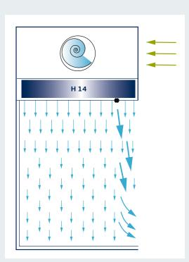
The WIBObarrier® economy safety workstation works with the tried-and-tested WIBObarrier® air flow principle. It is arranged for optimum product protection or protection of persons, products and the surrounding area, depending on the unit design.
