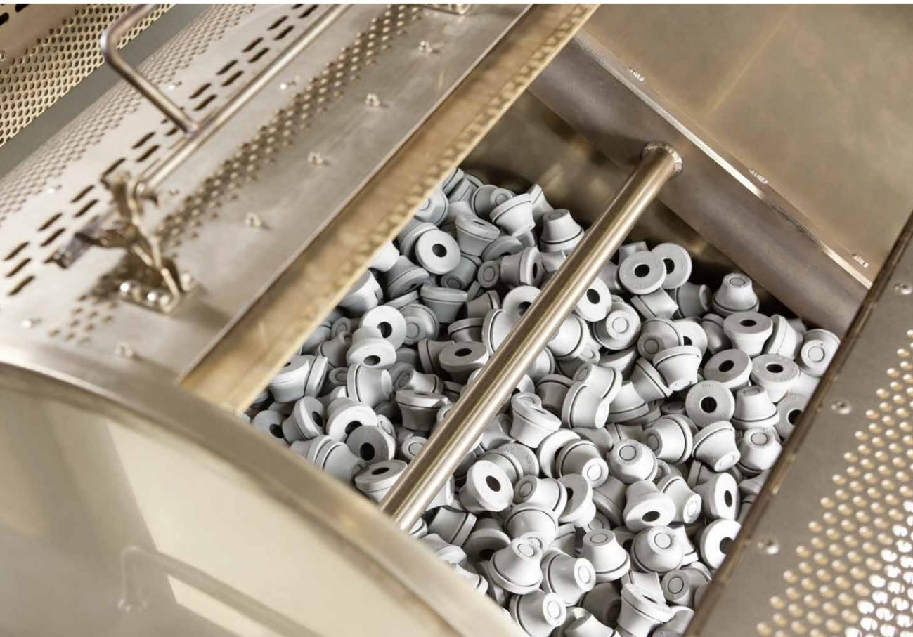
This is a huge advantage because starlim//sterner uses the oven to temper a wide range of products like seals and moulded parts for medical technology with different process times and temperatures. At the end of the process, an automatic message is created for the ERP system, enabling simple and comprehensive documentation of production.
