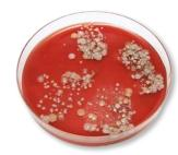
Sedimentation plate with bacterial contamination caused by air.
